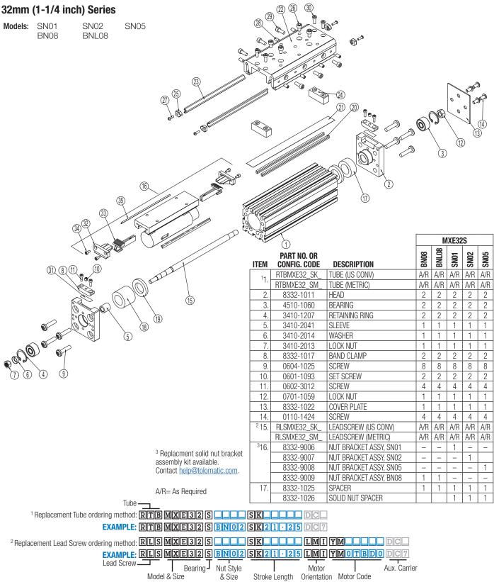
**Auxiliary Carrier Option Note:** If replacing a Lead Screw (6.), Tube (9.) or Dust Band (15.) on an actuator that has an Auxiliary Carrier, be sure to add "DC \_ \_ \_ " to the end of the configuration string when ordering. "DC" indicates the need for additional length and " \_ \_ " indicates the measurement of space between carriers (in inches [SK] or millimeters [SM] as indicated earlier in the configuration string).
