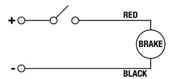
Figure 6.1: Fastest Engage / Disengage time, least protection
