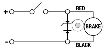
Figure 6.2: Increased Engage / Disengage time, best protection
