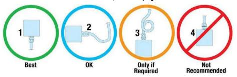
Figure 5.1: Recommended routing of ServoWeld cabling.
