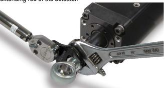
Figure 4.5: Hold thrust rod stationary using a wrench on the flats of the rod end when attaching accessories, linkages or load to the actuator. Two wrenches are used here: The crescent wrench prevents the thrust rod from rotating, the torque wrench will fasten the spherical rod eye option to the actuator rod end. Torque values provided in Table 4.1
