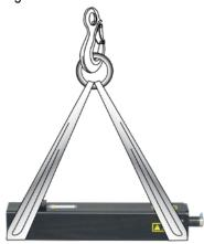
Figure 4.4: Use straps and winch to position heavy IMA actuator.
