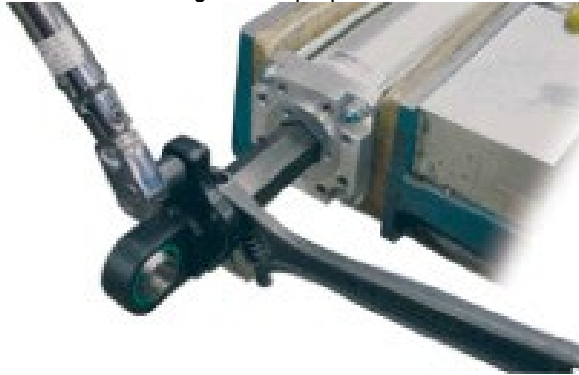
Figure 4.4: (SWA pictured) For hex rod, hold thrust rod stationary using a wrench on the flat of the rod when attaching accessories, linkages or load to the actuator. Use a torque wrench to tighten the interfacing rod end to the actuator threaded connection point. Torque values provided in Table 4.2.
